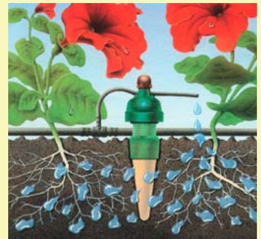
Above: Spare basket row. Directly below: As the soil dries out the valve opens to irrigate the growing media. As the media becomes moist, water passes through the walls of the cone, reducing and ultimately turning off the irrigation. Bottom: Blumat valve in operation. Note the Hydroton expanded clay.
