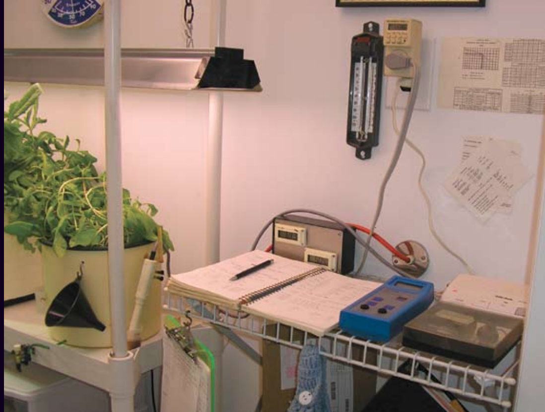
Larry's grow room is equipped with combination pH/EC meter, light meter, temperature/humidity indicators and programmable timer. There's also an intercom for communications within the house.
